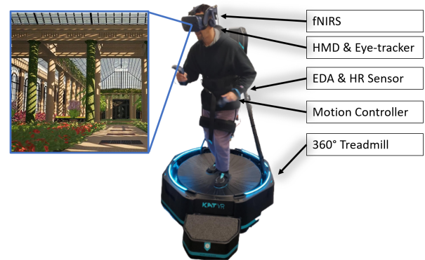
Figure 1. Kat Walk Treadmill and subject with VR HMD
