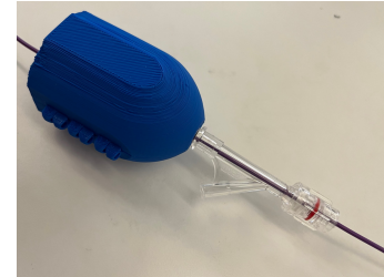
Figure 1: RHV O-ring housing with internal encoders
